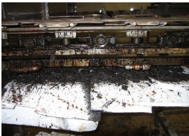
Carbon Debris removed before converting from Competitor's lubricant to Petrochem's by using CC-2208 FG Carbon Clean
